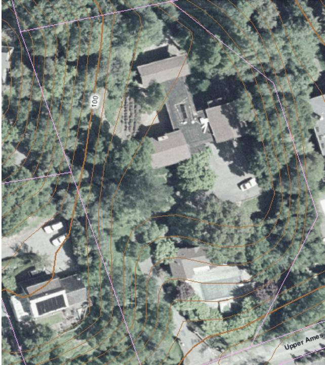
*It can be difficult to determine the slope of a lot when there are multiple slopes or the building is sited in a flatter area of the lot.*
