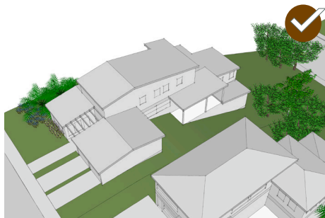
Design a building to respect and reflect the natural topography, especially in hilly areas.
