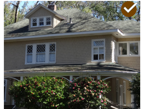
Establish a sense of human scale in the design of a building. The building above incorporates a one-story porch to convey a pedestrian scale.
