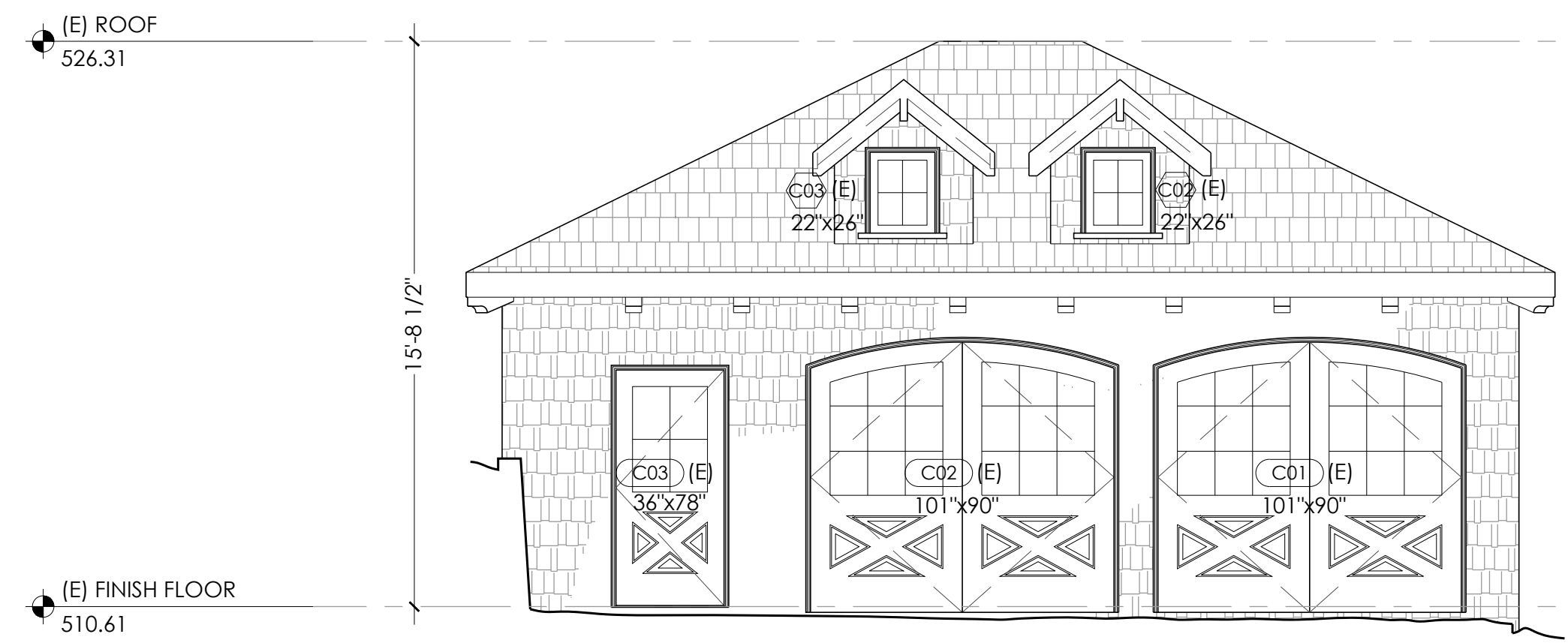
3 CARRIAGE HOUSE ELEVATION: SOUTH (NO CHANGE) 1/4" = 1'-0"
